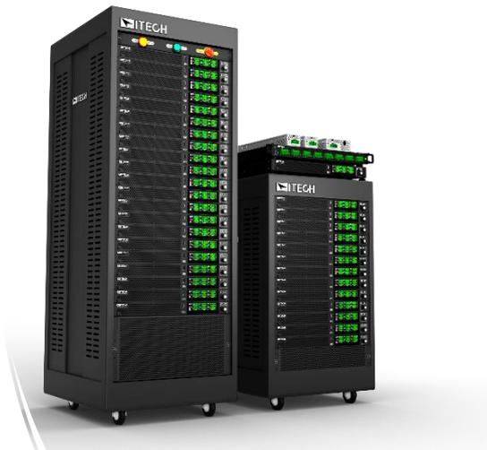
The IT2700 series Multi-channel Modular Power System offers ultra-high power density. The 1U chassis can accommodate up to eight 200W modules or four 500W modules. The modules can be bi-directional DC power supplies, unidirectional DC power supplies, or regenerative DC electronic loads. The modules support mixed configurations, synchronization, and can be connected in series
